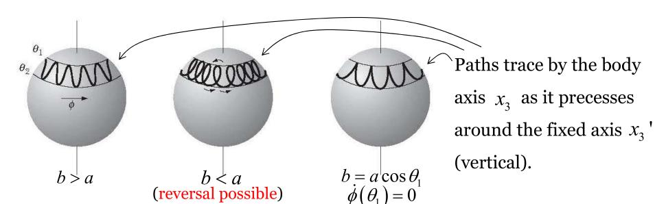
The precession rate of the body axis  $x_3$  is described by:  $\dot{\phi} = \frac{b - a \cos \theta}{\sin^2 \theta}$
