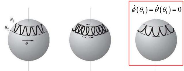
The last situation actually corresponds to the typical situation when the symmetric top is initially spinning about its body axis  $x_3$  fixed at a given direction  $\theta = \theta_0$  wrt to the fixed  $x_3$ ' axis. Then, the top is released.
