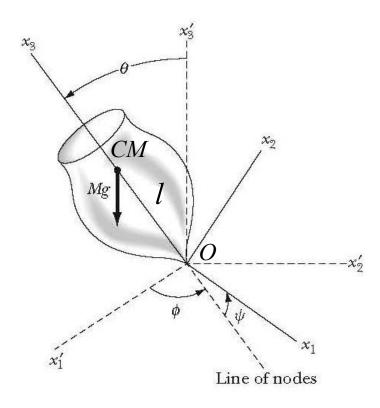
$$I_{1}\dot{\omega}_{1} - (I_{2} - I_{3})\omega_{2}\omega_{3} = N_{1}$$
